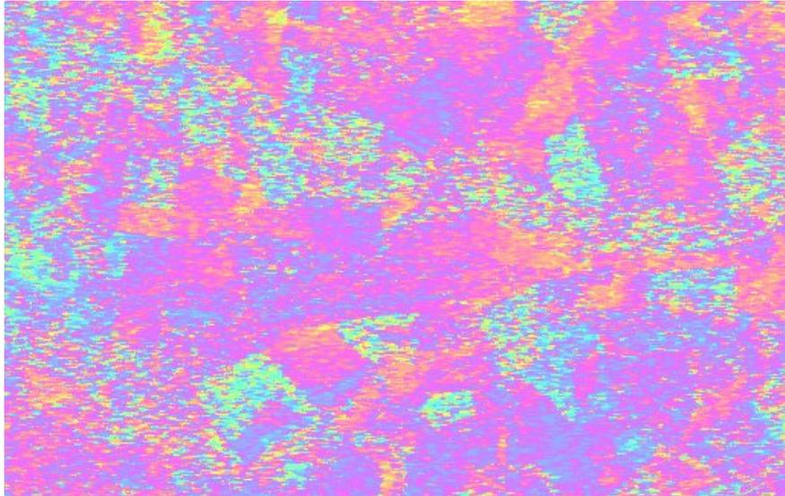
Figure 5.3: Three-pass deformation interferogram of the southern part of the scene. This area is out of the coal mines and therefore no deformations are expected here. Due to the fact that the "deformed" areas with different phase than their surroundings have sharp edges, we attribute the phase change to different farming activities at the fields.
